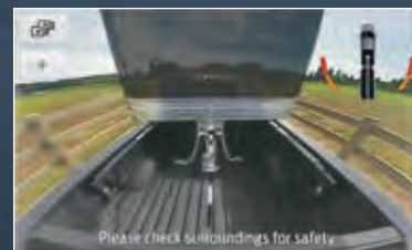
REAR CHMSL CAMERA VIEW The zoom feature of this view is particularly helpful when connecting a 5th-wheel or gooseneck trailer.
